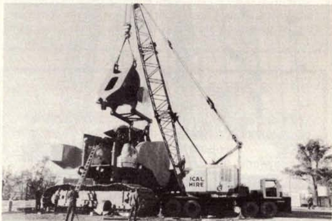
Lifting one of the heaviest components into position during the assembly of the 600-tonne Marion 204M face shovel at Lemington open cut mine in the Hunter Valley.
